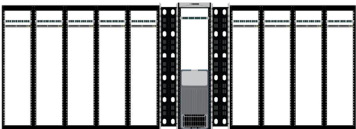
Bay Face of one 10 Racks row: 9xEDAS (Server Racks) and 1xHDA (MoR)
