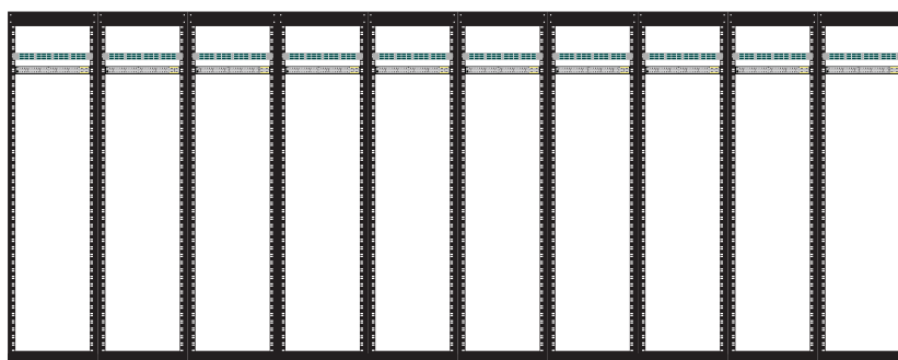
Bay Face of one row 10xEDAs (Server Racks) and 1xMDA
