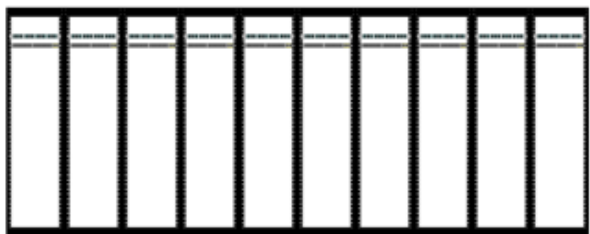
Bay Face of one 10 Rack row: 9xEDAs ToR (server racks) and 1xMDA
