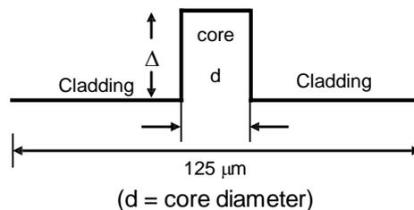
Fig.1 Refractive index profile, Dispersion Unshifted Single Mode Fiber
